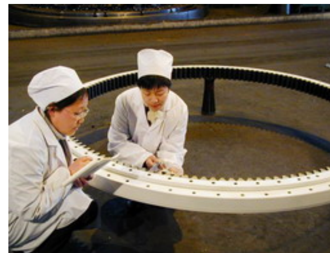
Extra-large wind energy bearing inspection
