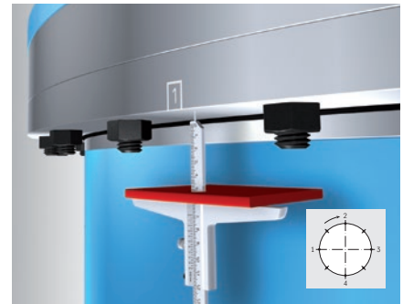
Figure 36: Basic setup for measuring the axial reduction with a depth gauge
